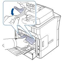
9. Return the lever, door, stopper, and guide to their original position.10. Close the rear cover. Printing automatically resumes.
